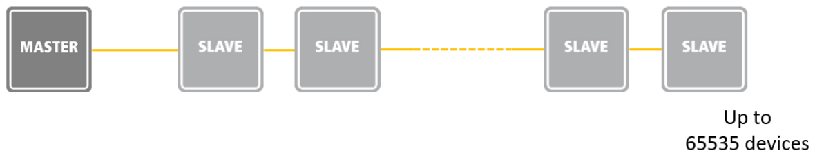
Figure 1: number of slaves on an EtherCAT network
