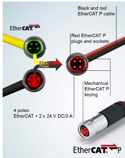
Figure 33: M8 P-coded connector and cable
